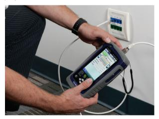
The world's most-advanced cable certifier is also the fastest Tier I fiber certifier. Not only can you save 30 minutes on every 150 CAT6A cables you test, you can now get fiber loss, length, pass/fail measurements in 8 seconds.
