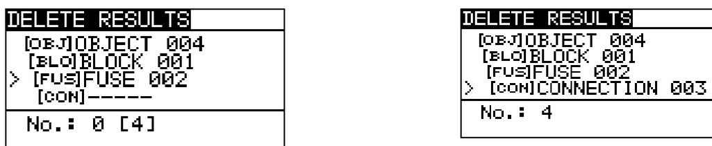
Figure 6.8: Clear measurements menu (data structure field selected)
