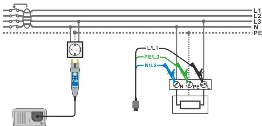
Figure 5.17: Connecting the plug commander and the 3-wire test lead
