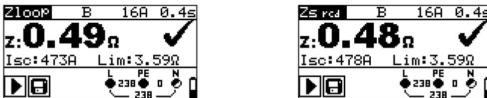
Figure 5.25: Examples of loop impedance measurement result
