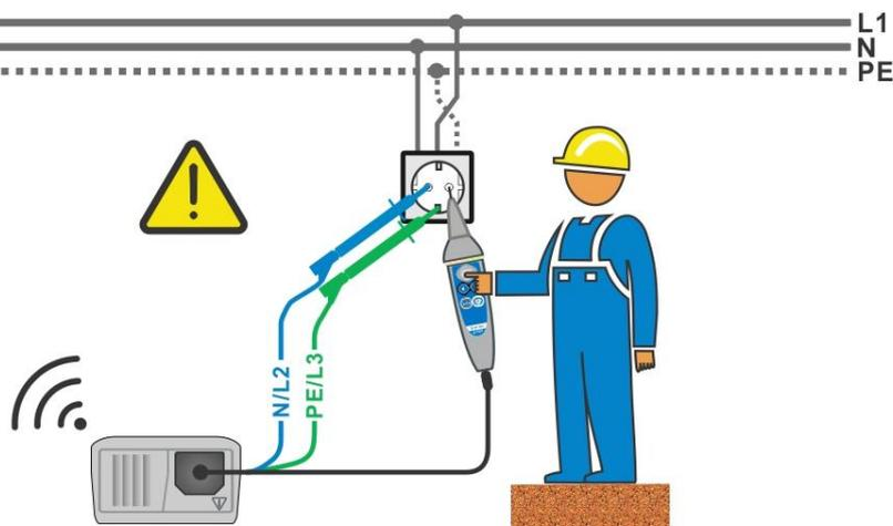
Figure E.5: Reversed L and PE conductors (application of tip commander)
