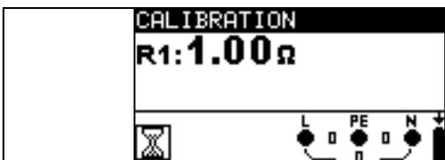
Figure 5.14: Results with old calibration values
