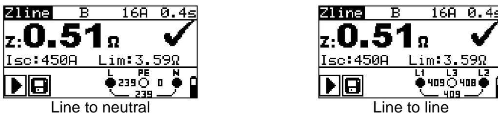
Figure 5.29: Examples of line impedance measurement result
