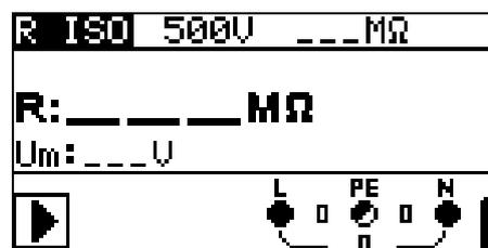
Figure 5.5: Insulation resistance
