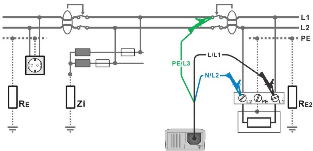
Figure D.3: RCD testing in IT system with bypassing RC
