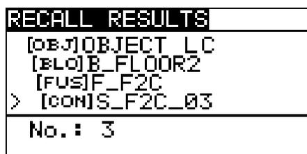
Figure 6.12: Example of menu with customized installation structure names
