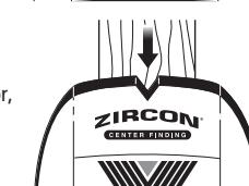
In cases of deeper studs (thicker walls), when the centre of the stud is located, only two bars will show on the Signal Strength Indicator and only the SpotLite® Pointer and middle segments of the Target Indication Bars will illuminate. If you still cannot locate a stud, try DeepScan® mode. Display will light green with the word "DeepScan" to indicate the mode.
